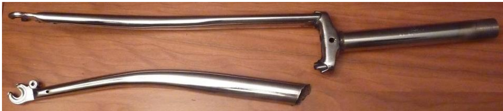
Figure 2. Bending failure of front fork
